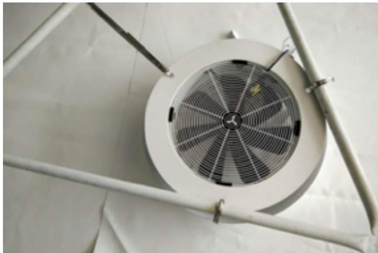
Securing the solar fan lid to the struts with metal fasteners.
