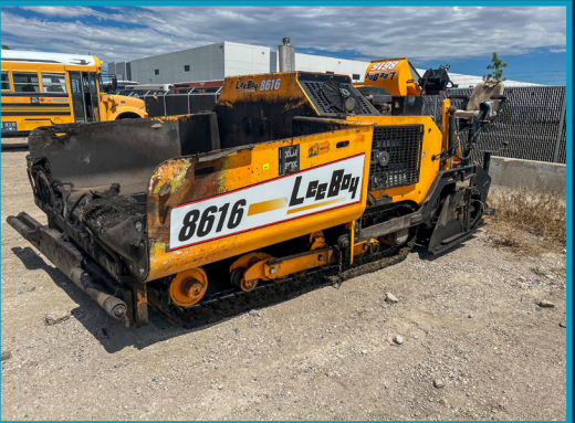
LEEBOY 8616 TRACK ASPHALT PAVER W/ 8' -15" SCREED
