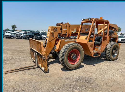
LULL 844C-42 4WD TELESCOPIC FORKLIFT, 8000 LB. CAPACITY
