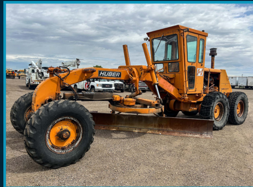
1960 HUBER D-1400 MOTOR GRADER W/ 14" MOLDBOARD
