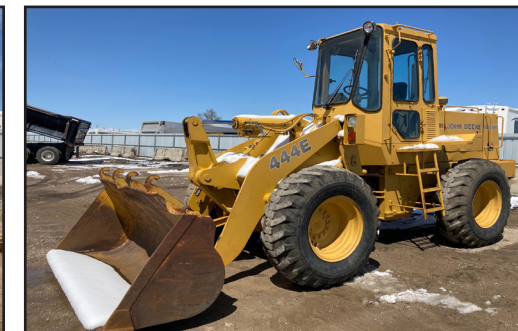
JOHN DEERE 444E WHEEL LOADER W/ 3RD VALVE
