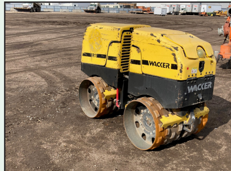
WACKER RT TRENCH COMPACTOR W/ LOMBARDINI DIESEL
