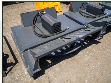
NEW 72 IN. HYDRAULIC BRUSH CUTTING ATTACHMENT TO FIT SKID STEER
