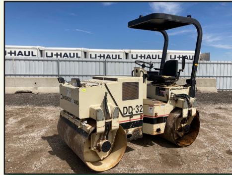
INGERSOLL RAND DD-32 DOUBLE DRUM ROLLER
