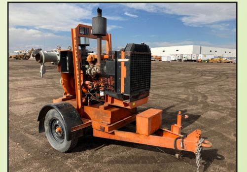
GODWIN 6 IN. TOWABLE DIESEL PUMP, COUNTY UNIT
