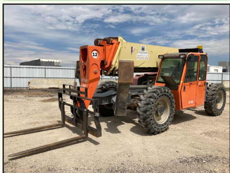
2011 JLG G12-55A TELESCOPIC FORKLIFT, 12,000 LB. CAPACITY
