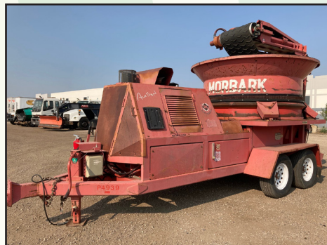
2003 MORBARK TOWABLE TUB GRINDER, CUMMINS DIESEL, CITY UNIT
