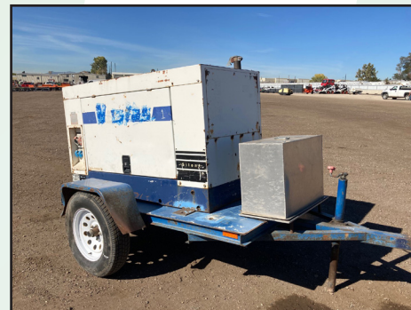
TOWABLE DIESEL GENERATOR, 22KVA
