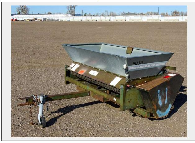
Vehicle Make Turfco Mete-R-Matic Vehicle Model III F120 Top Dresser Additional Features 60in, Pintle Hitch
