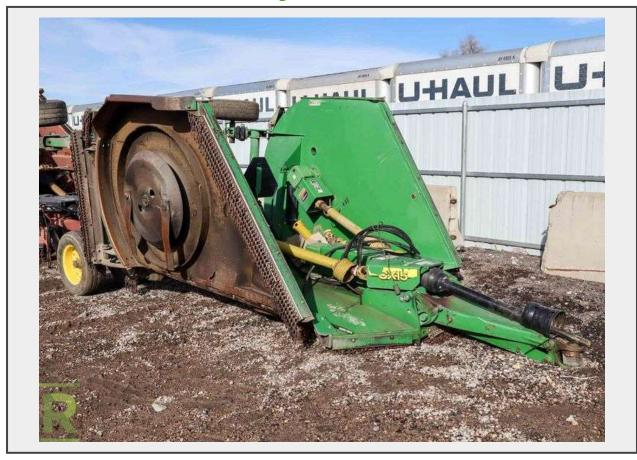
Additional Features 15' Mower Deck, PTO, Pin Hitch
