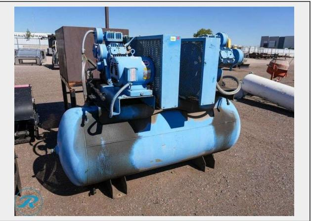
Additional Features 240 Gal, 460V, 3PH Electric, Dual Motor
