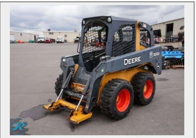
S/N 1T0320DATDG239566 Vehicle Year 2013 Vehicle Make John Deere Vehicle Model 320D Hour Meter 3471 Engine John Deere Fuel Type Diesel Additional Features Auxiliary Hydraulics Noted Issues No Bucket, Valve Body Stuck. Front Tire Size 12-16.5 Pneumatic Rear Tire Size 12-16.5 Pneumatic Unit # 877
