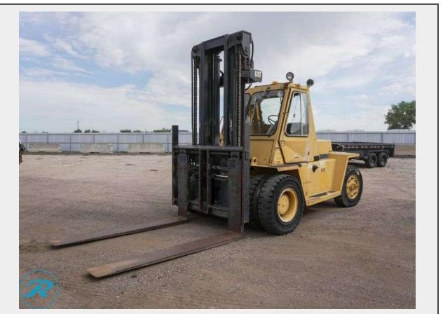
S/N 72Y02012 Vehicle Year 1991 Vehicle Make Caterpillar Vehicle Model V300B Hour Meter 4250 Fuel Type Diesel Additional Features 30,000 lb Capacity, 127" Lift Height, Fork Positioning, Enclosed Cab, Dual Front Tires, 8' X 12" Forks Noted Issues Coolant Leak Front Tire Size 12.00-20 Solid Rear Tire Size 12.00-20 Solid
