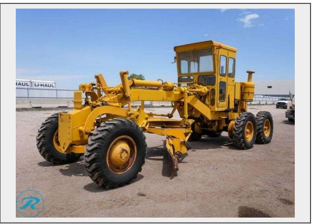
S/N GC-07825 Vehicle Make Galion Vehicle Model 118B Engine Detroit Fuel Type Diesel Additional Features 14' Moldboard, Front Scarifier Noted Issues Bad Clutch, No Brakes Front Tire Size 13.00-24 Rear Tire Size 13.00-24
